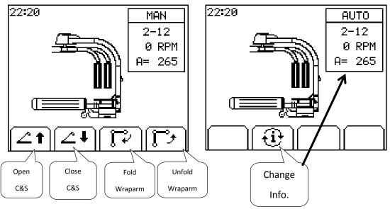
The box on the top right hand side of the screen can display additional operating and diagnostic information. It has three different displays. Pressing the (S2) (i) button changes the information displayed in this box, see below.
